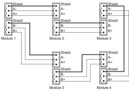
The diagram shows an example of the wiring for a closed VESDAnet loop, which is the recommended configuration. Remove the factory default A and B links from the VESDAnet sockets (C and D) prior to connecting the detector to the VESDAnet. It is recommended that 120 Ohm twisted pair cables (e.g. Belden 9841) be used for including the devices in the network, with a maximum length between devices of 1.2 km The polarity of the data wires must be maintained throughout the network.
