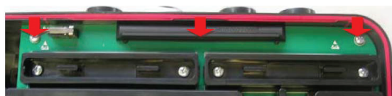
Figure 7: Main PCB fixing screws
